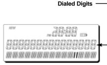
Figure 14 - Phonecell SX4D LCD Display
